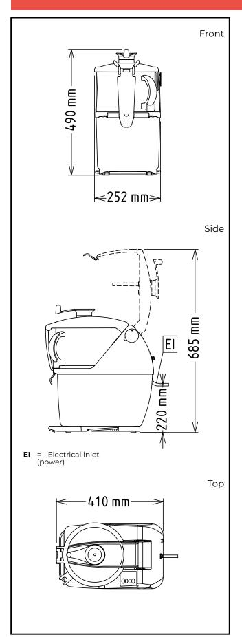
Electric Supply voltage: 600431 (DTRK45Y) 200-240 V/1N ph/50/60 Hz Electrical power max.: 1 kW **Total Watts:** 1 kW Capacity: Performance (up to): 550 kg/hour Capacity: 4.5 litres Key Information: External dimensions, 252 mm Width: External dimensions, Depth: 485 mm External dimensions, Height: 505 mm
